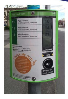
SmartGuide's InfoSmart MiniPID is a low-cost, real-time passenger information display designed for installation on existing street-side public transport stops. Shaped like a familiar timetable case, InfoSmart Mini PID shows the predicted arrival time for up to four routes. Back-to-back and multiple cases can be used for additional routes. A touch sensor in a fixed position plays the visual information in audio form, for maximum Disability Discrimination Act compliance.
